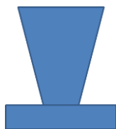
▲Reverse tapered pillars ▲Cross-sectional image
