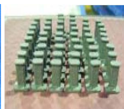
Net shape products of soft magnetic material with complex geometry
