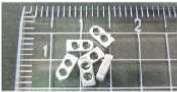
▲ MIM parts made from titanium
