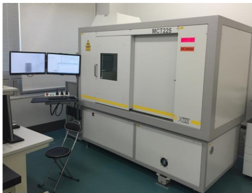
▲ Appearance of new X-ray CT scan system
